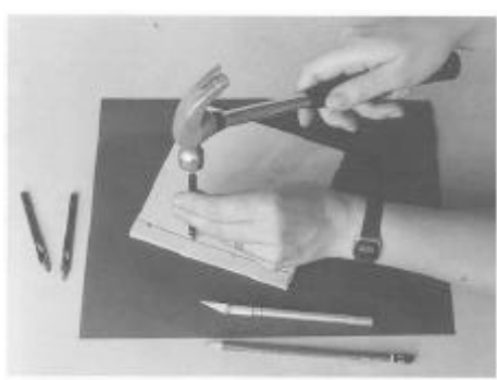
68 A leather hole punch is used on this stack of text pages for a Japanese stab or an album binding. A simple template marks the position of the holes. Photo: E. Lancaster.
